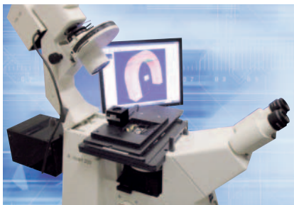
The microfabrication system operates on the basis of so-called "two-photon absorption". (Photo: Teem Photonics)
