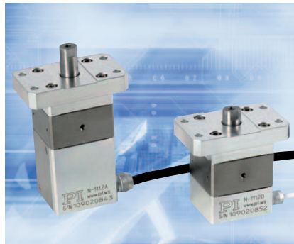
N-111 NEXLINE® Piezo stepping drives: high resolution, large travel and heavy loads. Piezo stepping drives combine piezo actuators with different motion characteristics. When driven in an appropriate way, both clamping and driving motions can be realized, the latter resembling the motion of a quadruped.
